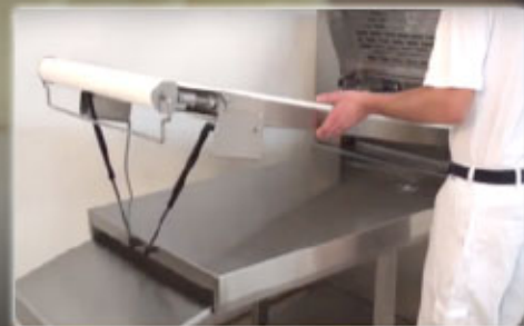
Pneumatic spring for safety covers and conveyor tables
