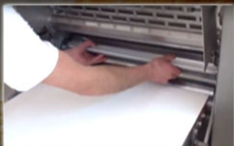
Scrapers can be removed and fitted without tools
