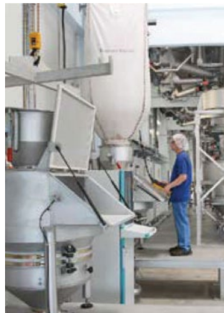
Segment-design, rectangular, indoor silos
