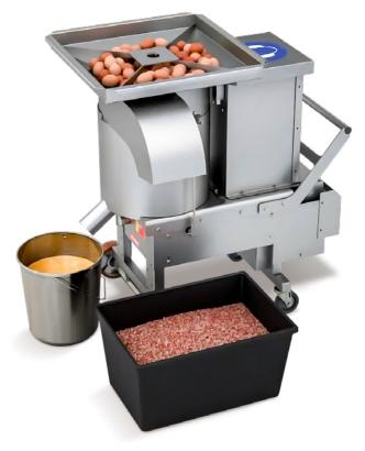
This centrifuge for eggs UDTJ-150 is a fully automatic machine. Made of stainless steel. It consists of the drive unit, hopper, tank, screw and sieve.
