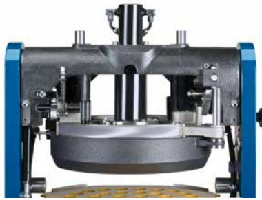
Low-pressure dividing system
