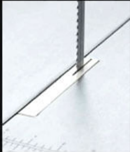
Precise saw blade guide
