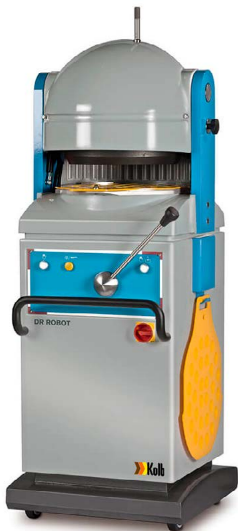
Interchangeable dividing disc
