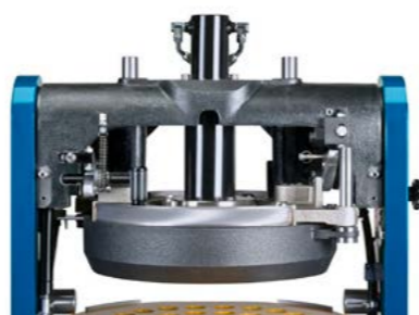
Low-pressure dividing system
