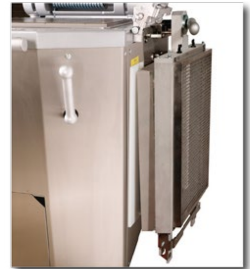
Right side grid and frame storage
